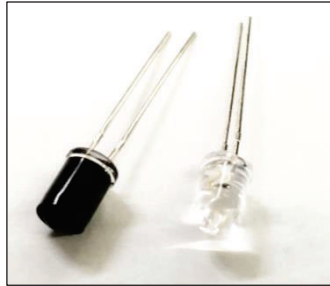
Figure 9-8. The PT334-6C phototransistor (right), wrapped in electrical tape (left).
