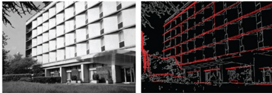
Figure 5.21 . This figure shows the straight lines detected (right) in an image (left) using Hough transform after edge detection. Note that some spurious edges can also be detected (as shown in the left) due to inaccuracies resulting from thresholding.
