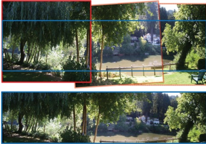
Figure 7.4 Three images (together) stitched together using homographic transformations to create a panorama (bottom). The red boundaries show the original images and the blue boundary shows a rectangular section cut off from the non-rectangular panorama.
