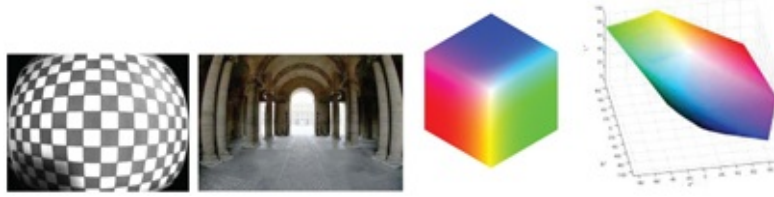
Figure 6.14 . Left two images show non-linear lens distortion that changes straight lines to curves. Right two images show the non-linear transformation (right) of a cubical 3D color gamut (left) during color management.
