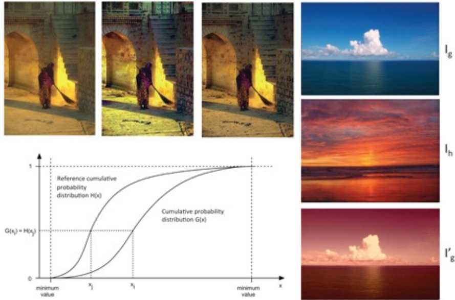
Figure 11.8 . The left three images on the top shows two different ways to handle color during adaptive histogram stretching. Left: Original image; Middle: Adaptive histogram stretching of each of the channels independently. Therefore hue is not preserved as is shown by the shift towards green on the door on top of the stairs and the shift to purple on the left side of the shadow and on the wall. Also notice that the shawl of the lady now has more saturated pink. Right: Adaptive histogram stretching applied only on the luminance channel resulting in a hue preserving contrast enhancement. However, whether it is more realistic or pleasant to look at may still be an arguable issue. For some, the more saturated pink and the higher contrast between sunlight and shadows may make the second picture aesthetically more appealing. The bottom figure shows the process of histogram matching. On the right, the histogram of I_g is matched with that of I_h creating I'_g that has the same look and feel as I_h .
