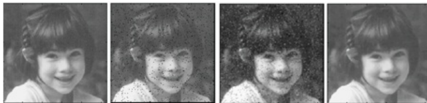
Figure 5.27 . This figure illustrates the effect of a median filter. From left to right: the original image; the original image with salt and pepper noise added to it; the noisy image processed using a box or mean filter; the noisy image processed using the median filter to provide an image almost identical to the original image.
