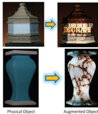
Figure 12.9 . Real objects (left) augmented with light projected from three different projectors to create spatially augmented reality objects (right).
