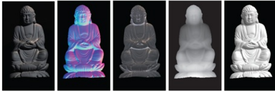
Figure 11.20 . From left: One of the input images; the recovered surface normals encoded by a RGB vector; the surface albedo; the reconstructed depth where depth is inversely proportional to the gray value; the same object relighted from a different virtual direction.
