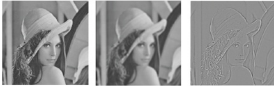
Figure 3.17 This figure shows the original image (left), the corresponding low pass filtered image (middle) that provides the basic shape of the object, and the high pass filtered image (right) created by subtracting the low pass filter from a delta that provides the details required to identify the face. The frequency contents of the right two images are complementary to each other and together create the entire range of frequencies present in the original image on the left.
