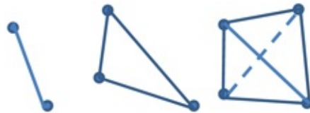
Figure 2.5 From left to right: The smallest 1D (line), 2D (triangle) and 3D (tetrahedron) simplex.
