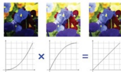
Figure 10.4 . On the left is a typical display gamma of 2.2. In the middle is the gamma of a capture device set to 1/2.2 to mimic the human eye. The result of putting this image on to the display is a linear response of input to output as seen in the right.
