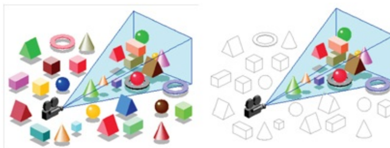
Figure 14.29 The figure shows the view frustum and all the objects in the scene (left) and then shows the objects which has been culled away by the view frustum culling by (right) using no color on them.
