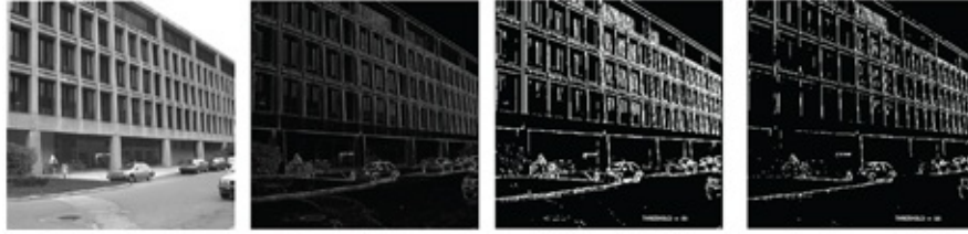
Figure 5.7 . From left to right: The original image, the gradient image obtained after applying the Sobel detector where the gray values denote the strength of the edges, the edgel binary image after thresholding with gray value of 64 and 96. Note fewer edges exist for larger thresholding value.
