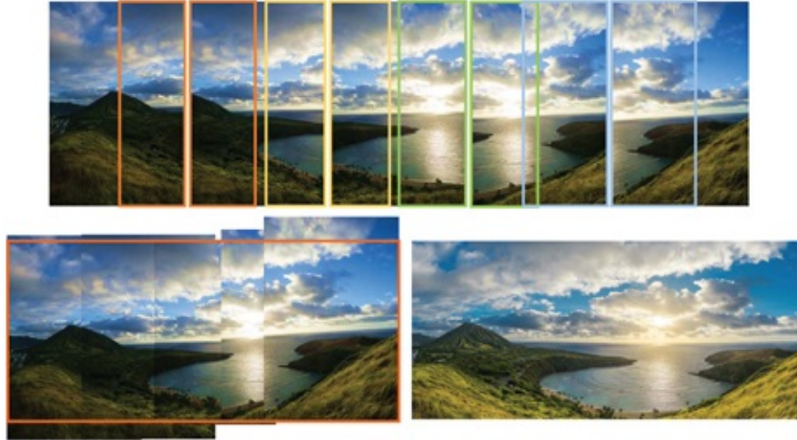
Figure 11.16 . Multiple contiguous images of a location are captured (top) with adequate overlap between adjacent images (shown by similarly colored rectangles). These images are then registered geometrically (bottom left) placing the overlap region exactly on top of each other. Finally, the regions coming from two adjacent images are blended using a blending function and the image cropped to form a rectangular panorama (bottom right).
