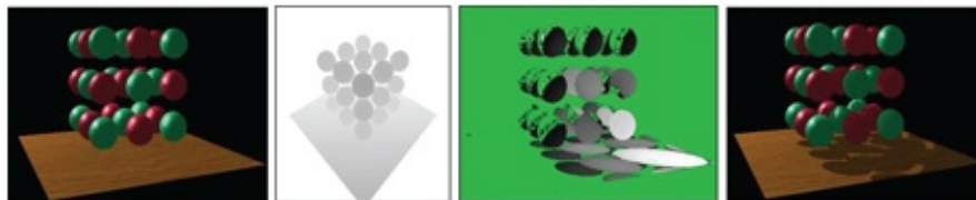
Figure 14.8 This figure shows pipeline for rendering shadows. From left to right: The 3 D scene rendered without shadows, the shadow map after the first rendering pass, the points in the framebuffer which are in shadow denoted by non-green values, these non-green pixel colors are attenuated to create the effect of
