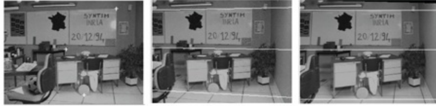
Figure 8.6 .This image shows the rectification. The left two images are unrectified and hence the epipolar lines corresponding to the features in the left image are not horizontal. The middle image is rectified to create the right image and the lines are now horizontal. The left and the right image together is called a rectified pair of Images.
