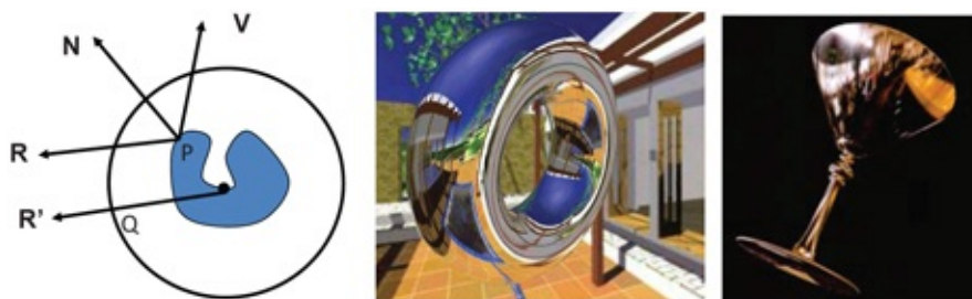
Figure 14.23 Left: The figure illustrates the environment mapping process for mapping the blue geometry enclosed in the spherical environment map. Q is the point mapped at P on the object. Middle: This shows a torus mapped using the cubic environment map in Figure 14.22 . Right: A wine glass mapped using the
