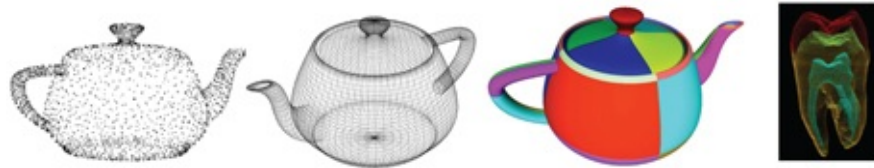
Figure 12.1 . This figure shows multiple ways to model an object. From left to right: We show a teapot modeled by a set of points, a mesh of quadrilateral polygons, a set of surface patches (each patch shown in a different color) and finally we show a volume representation of an object with tissue density values at every volume location which can be used to visualize the tissue density as transparency values (mapping least dense to transparent and most dense to opaque).
