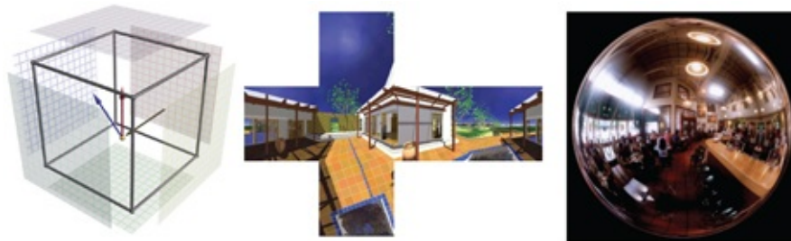
Figure 14.22 This shows a cubic and spherical environment map. The cubic map is shown unfolded (middle) and is generated by using a 6-pass rendering each rendering a face of a cube (left) seen from the center of the cube. The spherical map (right) is generated from images of a cafe taken using a fish-eye lens camera.
