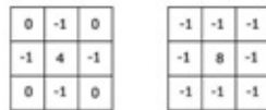
Figure 5.12 . The Laplacian operator considering only four perpendicular neighbors (left) and considering all eight neighbors (right).
