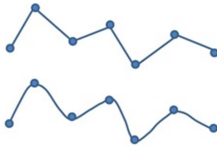
Figure 2.1 This shows the assumption of smooth transition between samples in interpolation and how it can be modeled differently. Top: Linear; Bottom: Non-Linear.
