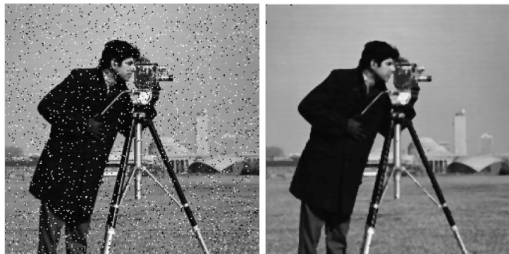
Figure 2.10: Image with salt and pepper noise (left) and the result of the median filter (right).
