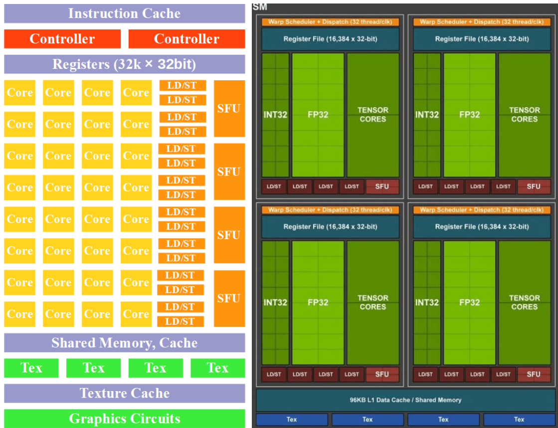
Figure 16.4: The SMs of the Fermi (2010, left) and of the Volta (2017, right) architectures.
