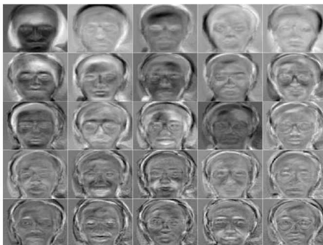
Figure 4.13: The significant principal components of a database of faces (i.e. face-like images). Note that these images result after subtracting the mean of the pixels.
